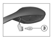
• Install bulb 3 in bulb socket.
